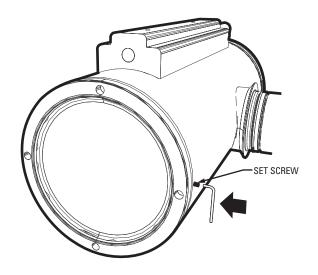
Figure 4. Loosen Set Screw
